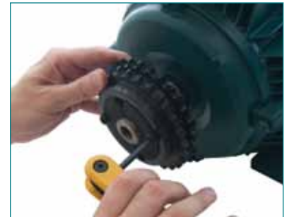
TIGHTEN SCREWS ALTERNATELY
