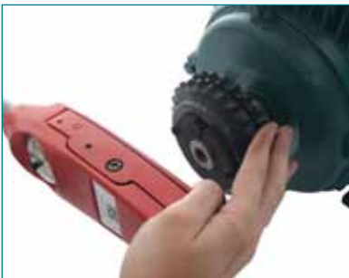
TIGHTEN SCREWS TO THE CORRECT TORQUE SETTING
