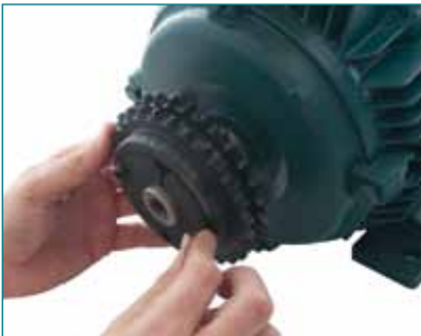
TIGHTEN SCREWS FINGER TIGHT
