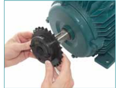
INSERT SCREWS AND LOCATE ON SHAFT
