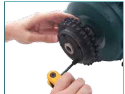
REMOVING A TAPER LOCK BUSH
